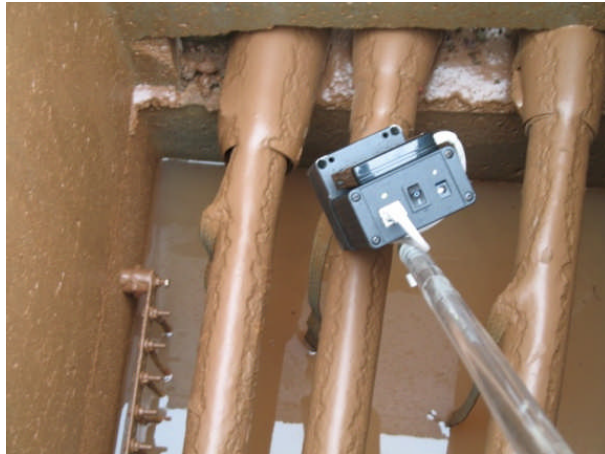
Example of measurement on a cable joint (joint end).
