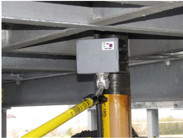
Detail of a measurement on an outdoor termination (cable sheath).
