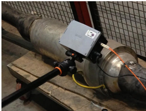
Example of measurement on a cable joint (screen earth).
