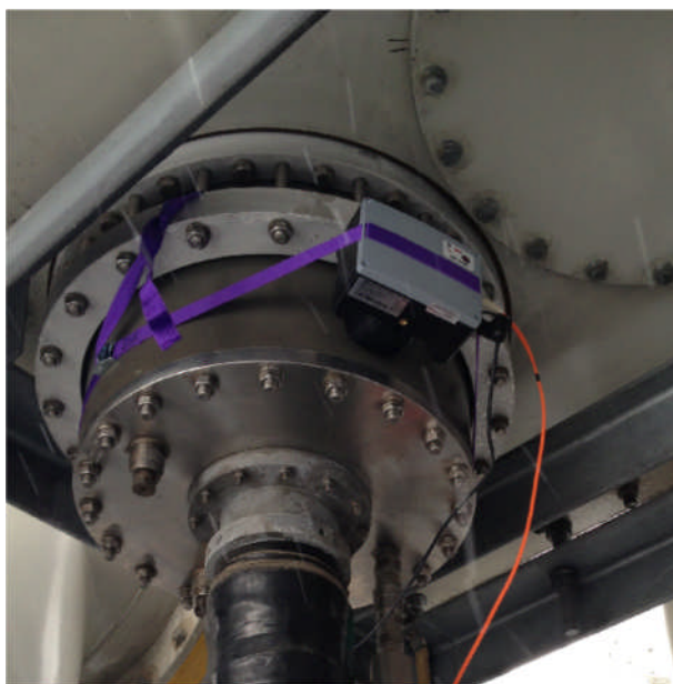
Example of measurement on a GIS termination (insulator ring).
