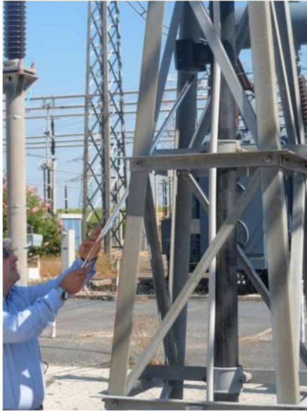
Example of measurement on an outdoor termination (termination earth cable).
